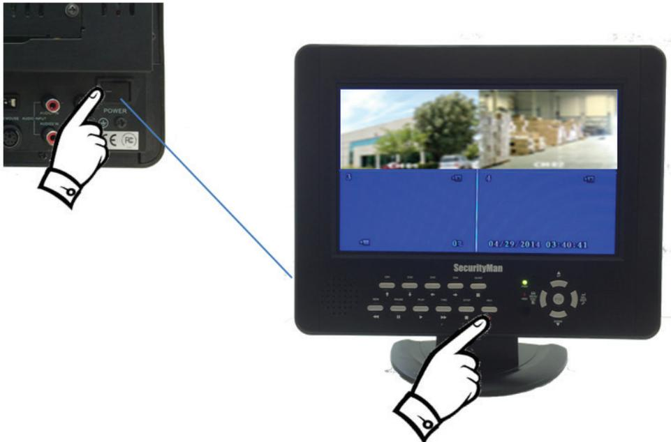
To begin recording, simply turn on the DVR by switching the DVR's On/Off button (located on the back of the DVR) to the ON position. The systems start up screen will be displayed for a few seconds and switch to a live view of all the cameras that are connected. At this point, all you have to do now is press the "REC" button located on the front of the DVR to begin recording.
