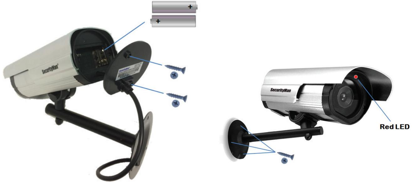
Using a Philips head screw driver, remove the back cover of the SM-3802 (dummy camera) and insert 2 AA batteries (not included). After inserting the batteries, re-attach the back cover and secure the camera with mounting screws provided.
